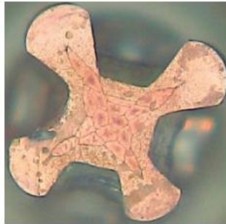
Uneven Crimp and Wall Thickness
