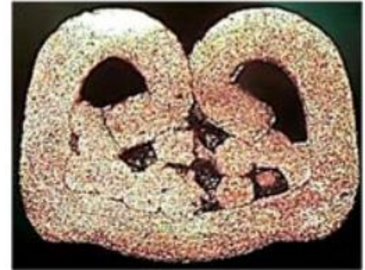
Crimp Too Loose and Void on Both Sides
