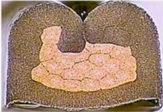
Uneven Crimp and Wall Thickness and Flash on Both Sides
